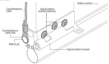
NEVER LOOSEN FASTENERS ON BOTTOM FIXTURE. USE CAUTION WHEN TIGHTENING FASTENERS BECAUSE BOTTOM FIXTURE IS UNDER HIGH SPRING TENSION.
