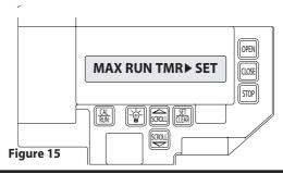
**CAUTION:** The MID-STOP feature must be turned off in order to properly set the Max Run Timer.
